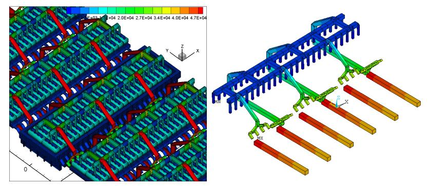
Improved RCC busbar network concept with alternating risers
