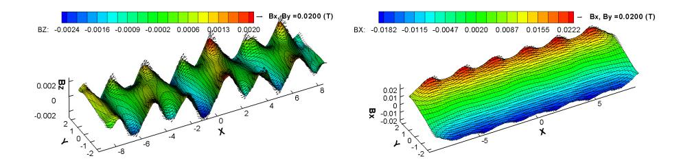
Corresponding  $B_z$  and  $B_x$  magnetic field components
