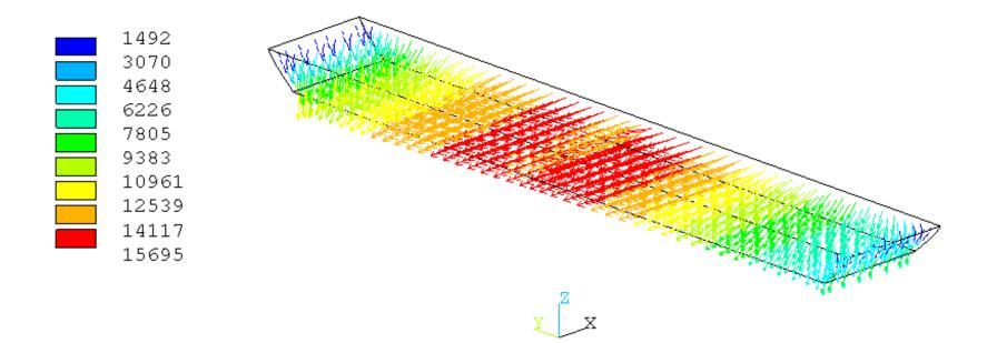
Thermo-electric model metal pad current density
