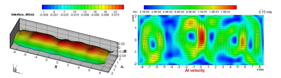
Corresponding steady-state bath-metal interface deformation and steady-state metal pad flow velocity field
