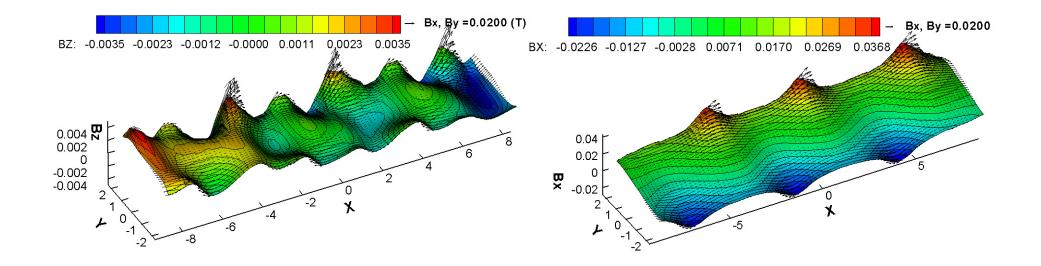
Corresponding  $B_z$  and  $B_x$  magnetic field components
