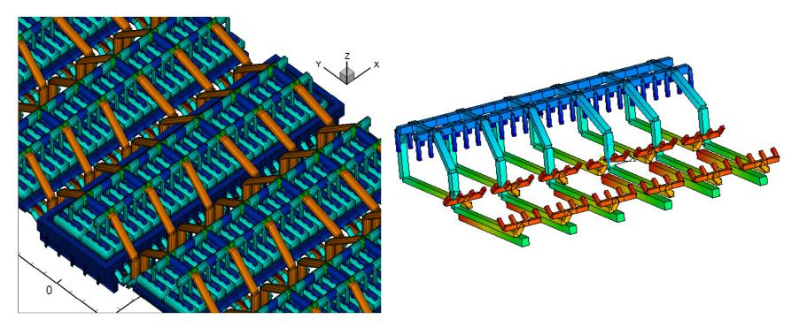
Original RCC busbar network concept with downstream risers
